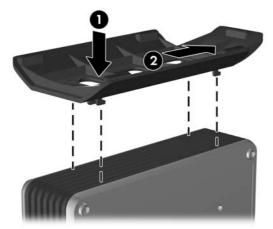
Figure 1-4 Installing the stand
